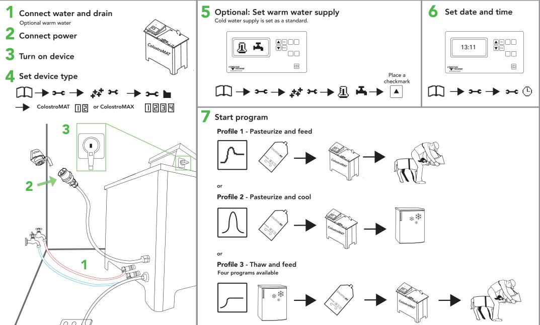
This checklist is based on the basic equipment of the ColostroMAT. Potential extensions aren't listed separately. For detailed information and valid warnings as well as safety instructions refer to the instructions manual. (Status 01/2023)
